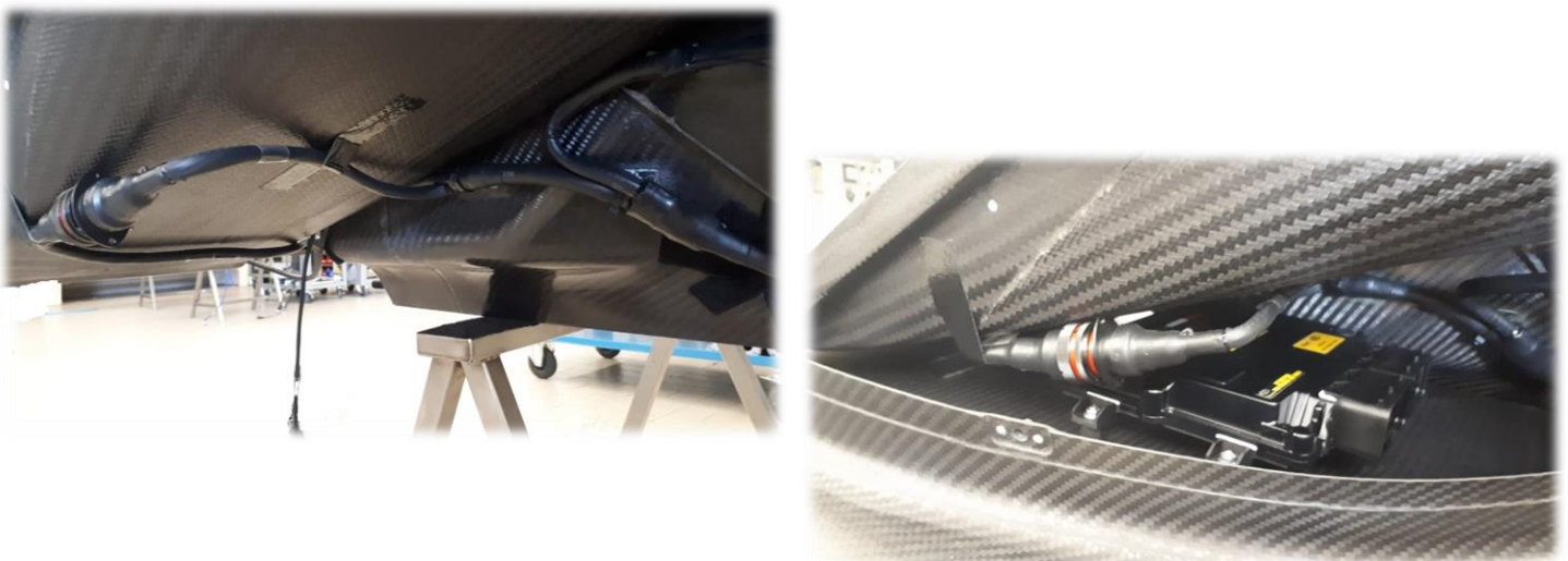
Fig.2,3: junction loom, suggested installation on the chassis.
