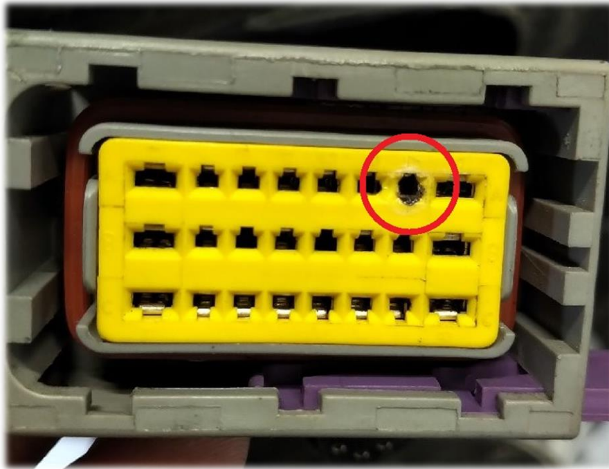
Fig.4: PIN 7A failed, chassis loom side.
